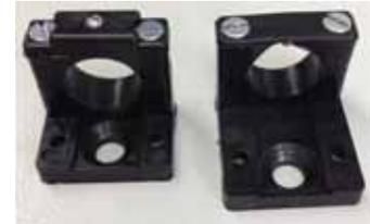
The long swivel fixture is meant for the side with the M12 connector.
