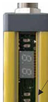
The red and yellow LEDs flash about once a second in blanking modes 3 – 11 to indicate reduced resolution or floating blanking.
