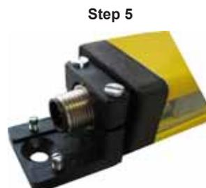
Fasten the long swivel fixture via the connector's M12 nuts.
