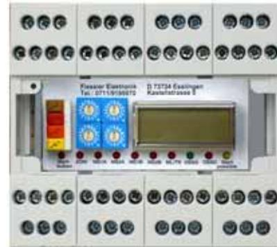
**BLPG:** Programming unit for BLCT blanking functions
