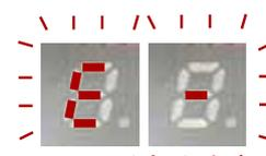
If you hold down the button for 2 seconds or longer, the currently displayed operating mode is saved and remains solidly lit on the display.
