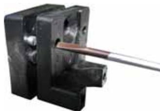
The adjustment screws can be turned inside the through-bores.
